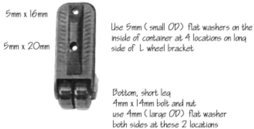
The preferred orientation of the fasteners is with the heads of the screws on the inside of the container and the locking nuts on the outside, however that fastener orientation requires a 5mm metric socket to tighten the nuts. If you don't have a 5mm metric socket, insert the screws from the outside and hold the nuts on the inside with pliers while you tighten the screws.
